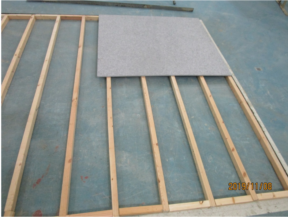
Figure 3 – Specimen partially installed over D-50 mounting materials
