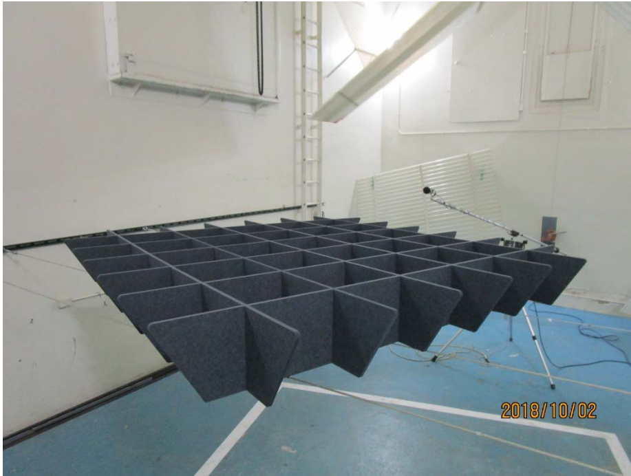
Figure 1 - Specimen mounted in test chamber
