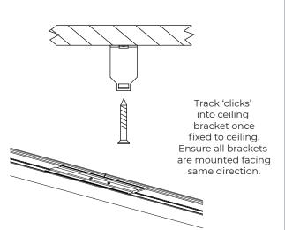
**3** Slide track onto mounted brackets (A) and secure end caps onto track ends (B)
