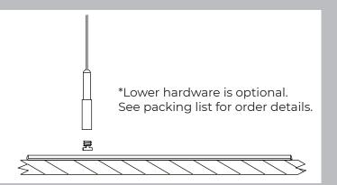
**6** Mark and drill pilot holes for Ezo Clamp on WZD
