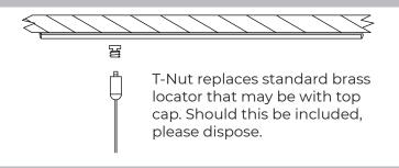
**3** Install the suspension track on the ceiling and floor\* using substrate appropriate fasteners (not included)
